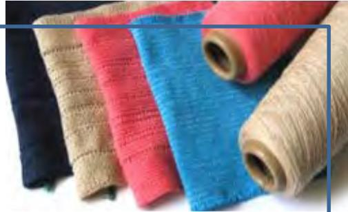
80% cotton yarn made from recycled cotton, obtained through a process that uses the processing waste of pretreated cotton items
