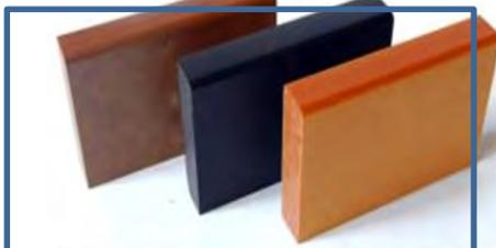
Panel obtained from cellulose fibres thermo- bonded
