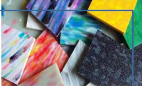
Material deriving from the recycling of HDPE packaging for detergents
