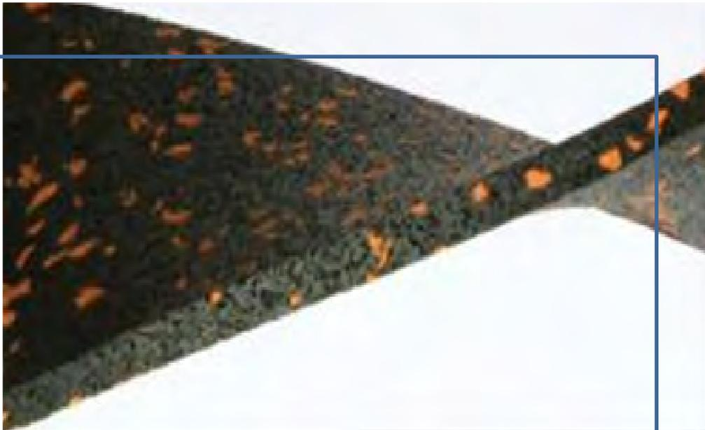
Material made of black SBR rubber granules recycled from tires and coloured EPDM rubber granules.
