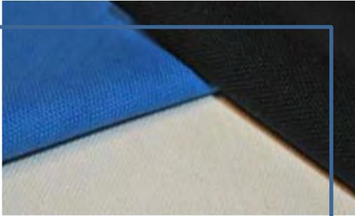
Fabric made of 100% recycled cotton from weaving scraps, threads and cut-outs
