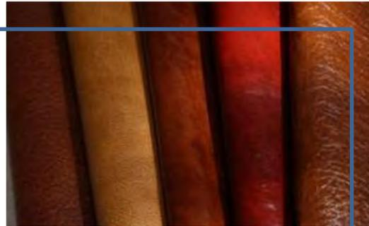
Fabric made with pulverized leather waste and used to reinforce a polyurethane fabric base
