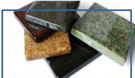
Material made of recycled paper through a particular process that allows you to use any type of paper
