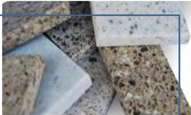
Material composed of 70% natural stone powder, partly recycled, from acrylic resin and natural pigments.
