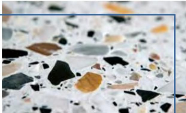
Material consisting of pebbles or recycled stone splinters and glass and mother-of-pearl splinters bound with a Portland cement base
